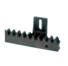
400CN Steel core, fibreglass reinforced, 22x22 nylon rack (Module 4, max 800 kg)
